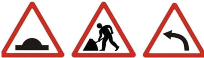
Fig. 2 Cautionary sign: hump ahead, men at work and left hand curve
