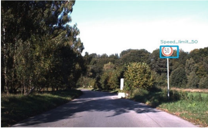
Fig. 14 Speed limit 50 sign board detection
