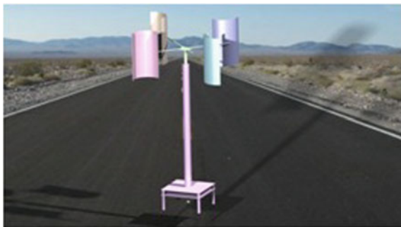
Fig. 3 Isometric view of 3D C-Type VAWT
