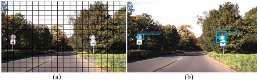
Fig. 9 a Grids formed on input image, b Bounding boxes formed for the grid cells
