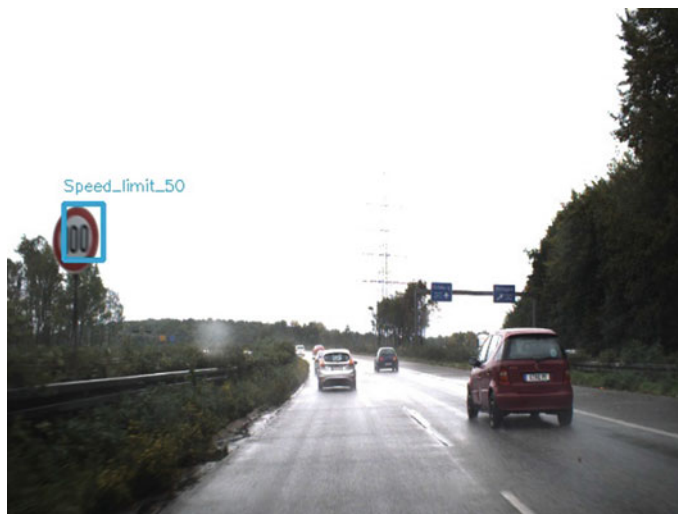
Fig. 20 Speed limit 100 detected as speed limit 50
