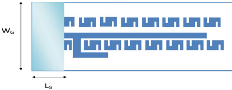
Fig. 5 Ground plane view of dual-band antenna with slotted EBG structure
