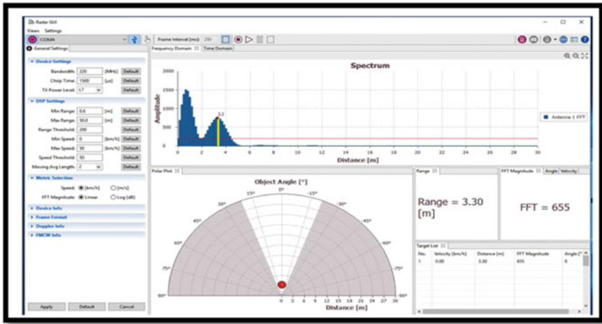
Fig. 8 Radar Obstacle map visualizer and SW development environment
