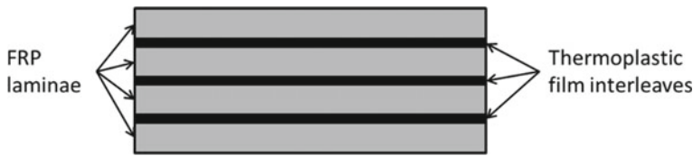
Fig. 9 Schematic of FRP laminate with thermoplastic film interleaves
