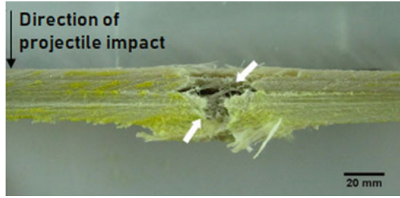
Fig. 8 Fibre breakage (Ávila et al. 2011)
