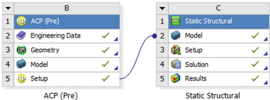
Fig. 8 Schematic view of static structural for hybrid laminate composite
