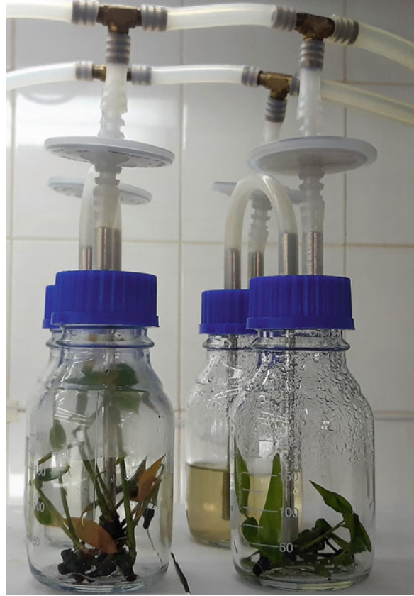
Fig. 9.5 Temporary immersion bioreactor (TIB) for bamboo propagation. Credits: Alzerina Kene Benmuyal Vieira and Palloma Sales de Assunção
