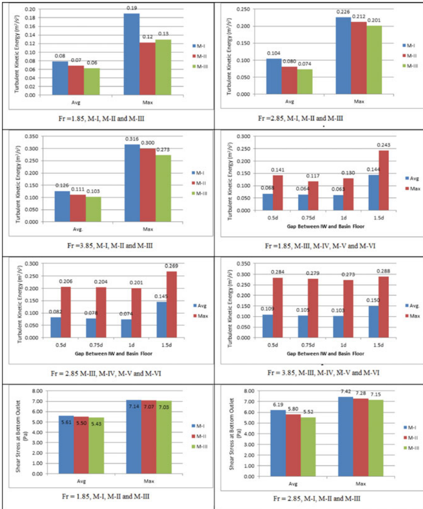
Fig. 5 TKE, WSS, and the change in KE and SE between inlet and outlet for different models (M-I to M-VI) at different Fr (i.e., 1.85, 2.85, and 3.85)
