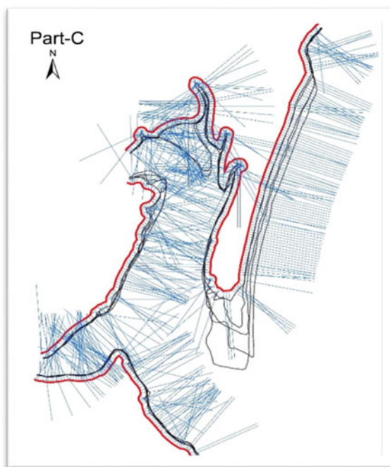
Fig. 16 Part C transects on baseline intersecting shorelines
