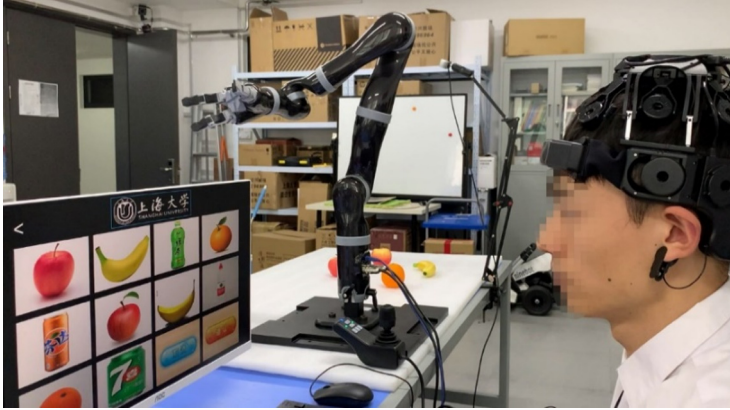
Fig. 4. Brain-controlled robotic arm experiment diagram
