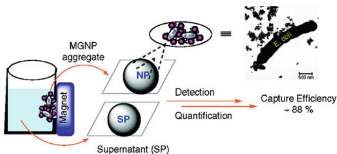
Fig. 9 Illustration of magnetic glycol nanoparticle (MGNP)-based system for the detection and separation of E. coli . Adapted from Ref. [110]. Copyright obtained from American Chemical Society 2007
