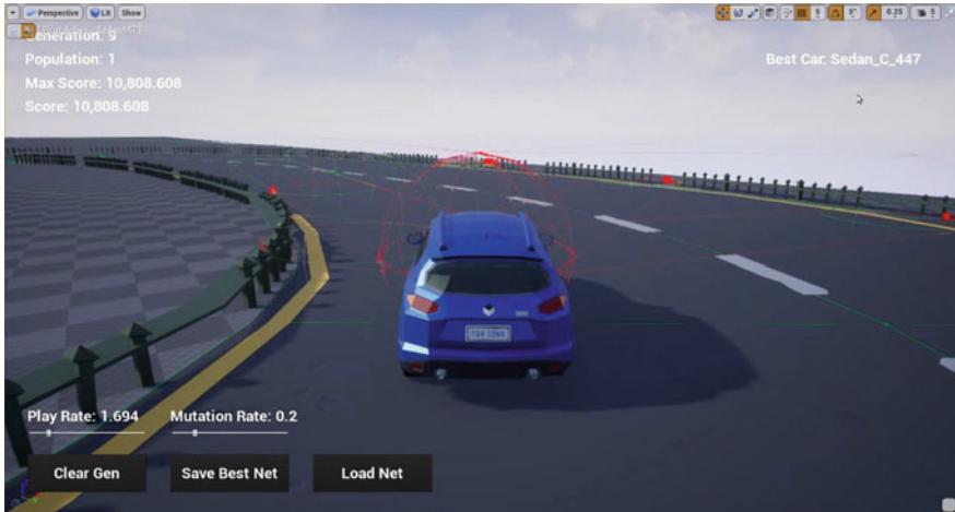
Fig. 6 Neural net has decided to stick to the left lane on the road through sheer randomness which can be nurtured by altering the fitness function
