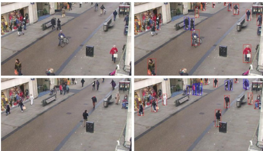
Fig. 5 Experimental results—blue boxes being high risk while red have been marked as safe
