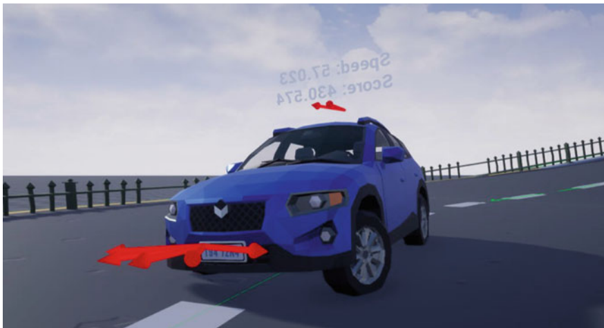
Fig. 7 Neural net has learned how to countersteer and control the car on the onset of oversteer
