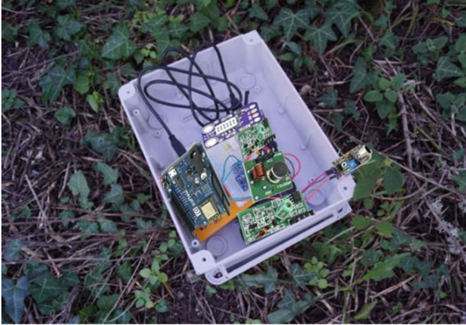
Fig. 20 Field testing of WSN node
