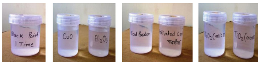
Fig. 6 Distilled water samples obtained from solar distillation units with different absorber coatings
