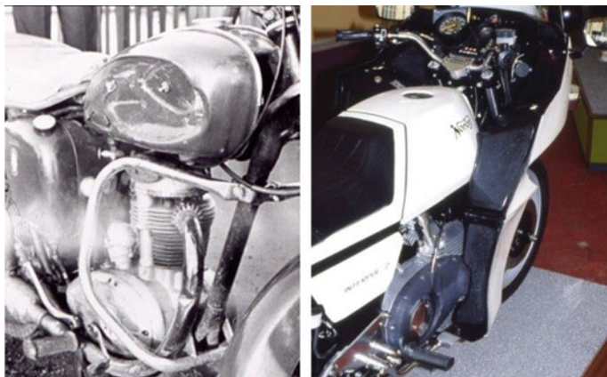
Fig. 10.6 Crash bar causing lower limb injury and an energy-absorbing fairing to protect the legs
