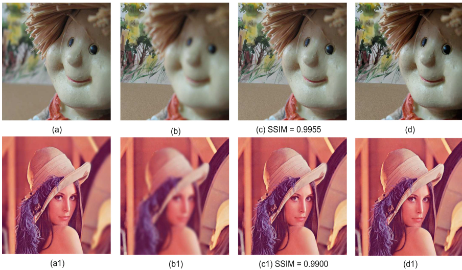
Fig. 8. Performance on artificial images: (a),(a1) Focus on Foreground; (b),(b1) Focus on Background; (c),(c1) Fused by the proposed algorithm; (d),(d1) Groundtruth image
