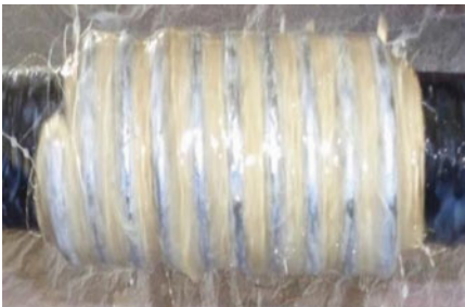
Moulded fibres on spring die after applying the epoxy resin
