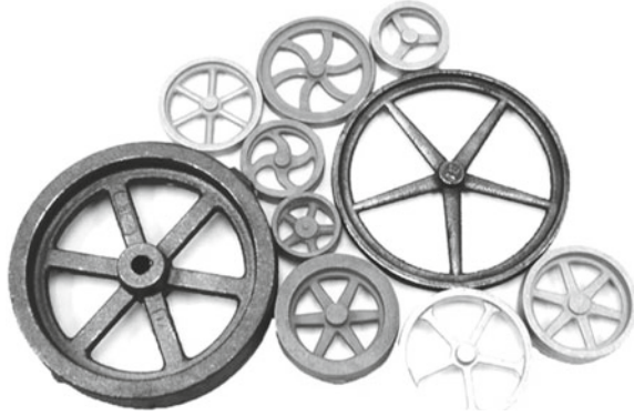
Fig. 1 The typical casting of different shapes of a flywheel
