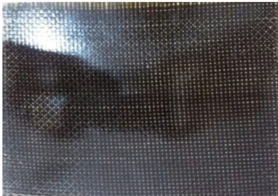
Fig. 1 KFRP-BFRP hybrid fiber composite specimen
