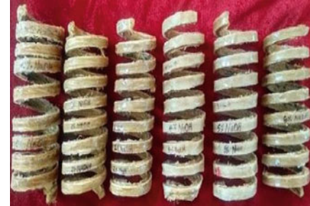
Fabricated spring of varying NaOH treatment level
