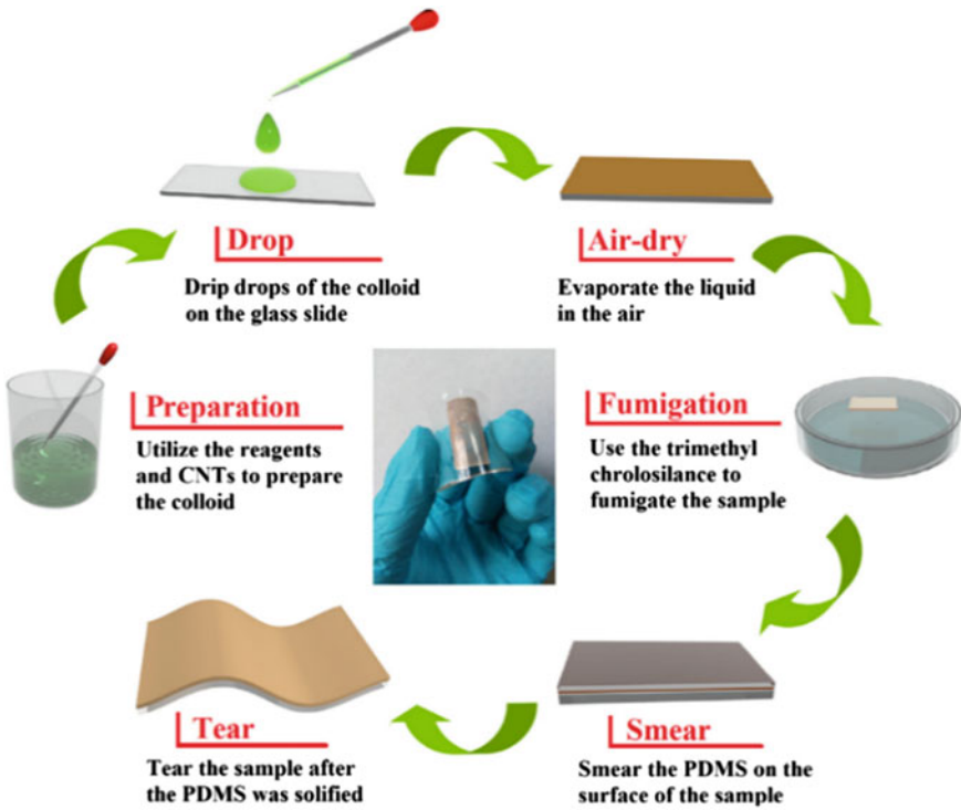
Fig. 12 CNTs/PDMS strain sensor fabrication process which is modified using silver nanoparticles. The as-prepared product is illustrated in the center. Reprinted with permission from [116]. Copyright © 2015, Elsevier
