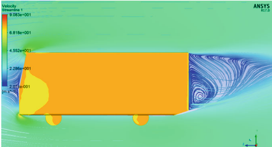
Fig. 12 Baseline model velocity contour at 120 kmph
