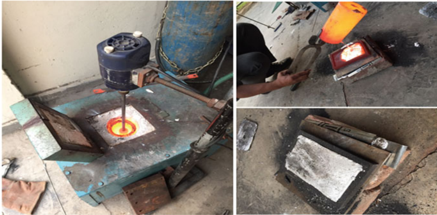
Fig. 1 Stir casting setup and operating processes
