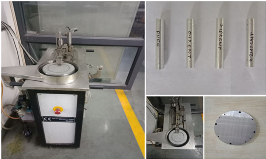
Fig. 2 Pin-on-disk setup with samples and disk
