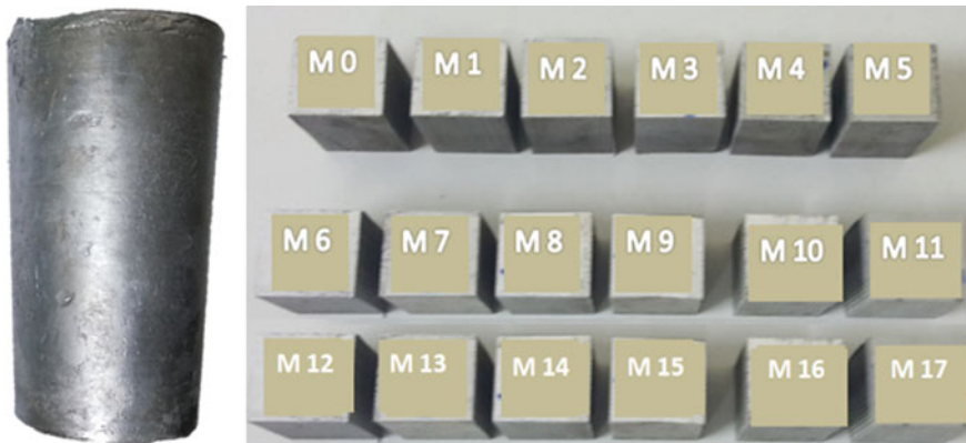
Fig. 3 Billet casting and samples was cut by CNC wire-cutting machine
