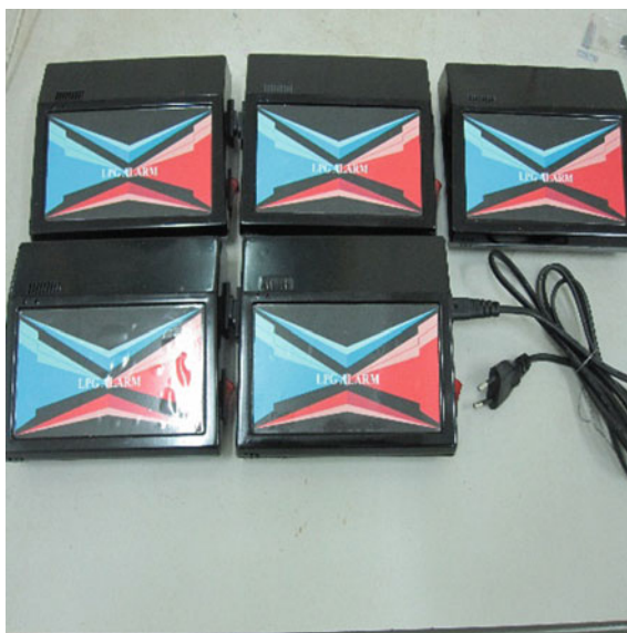
Fig. 10 LPG-leak detection device
