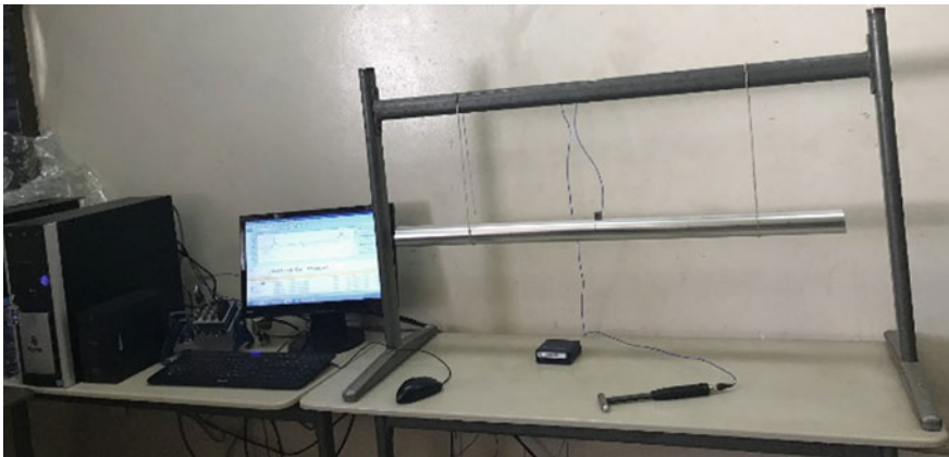
Fig. 2 Used experimental setup for the dynamic analysis of the aluminum pipe [17]
