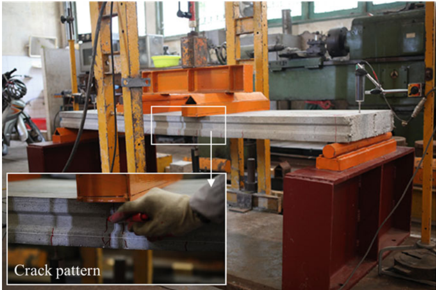
Fig. 4 Slab deformation and crack pattern
