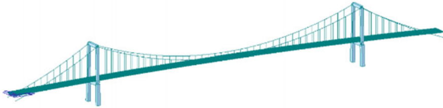
Fig. 8 3D FEM model Thuan Phuoc Bridge [5]
