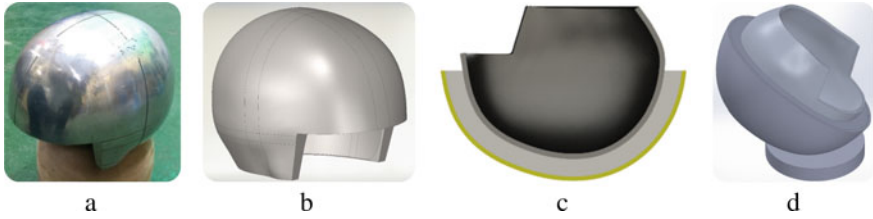
Fig. 6 The practical head form (a), 3D scan model in Solidworks (b) a cross-section view of the wear of helmet on the head form (c) and a fully assembled model with a flat anvil (d)
