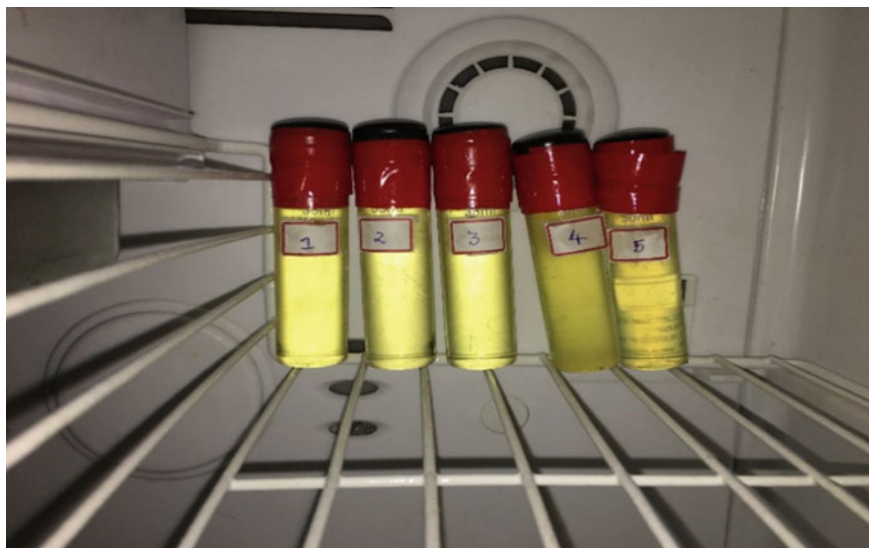
Fig. 6.5 Representative blends of diesel–ethanol with 10% n -butanol kept at 5 °C after 20 days
