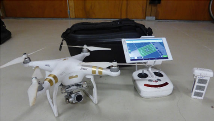
Fig. 27.3 Main components of a drone system: Drone, remote control, a ground control station (tablet) and drone battery. Image courtesy ( https://www.edx.org/course/drones-for-agriculture-prepare-and-design-your-drone )
