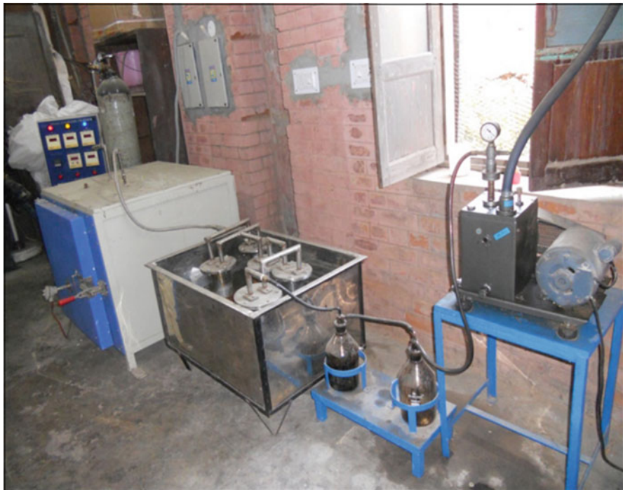
Fig. 11.3 Electrically operated temperature controlled biochar maker. Source: Purakayastha et al. (2016a)
