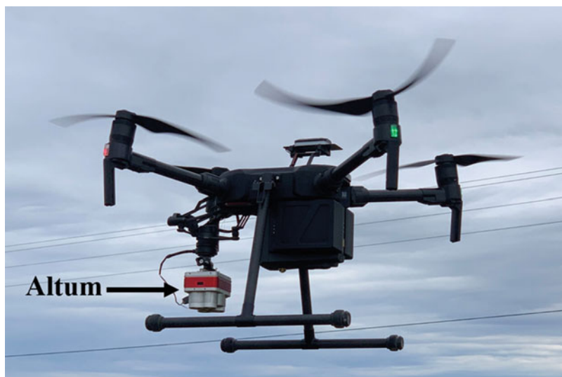
Fig. 28.3 A MicaSense® Altum (MicaSense, Seattle, USA) multispectral sensor mounted on a DJI Matrice 200 (DJI, Shenzhen, China) UAV. The sensor collects data in six bands (red, green, blue, red-edge, near-infrared, and thermal) simultaneously
