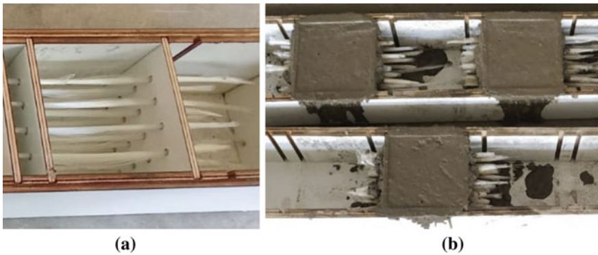
Fig. 2 Preparation of luminous concrete; 2(a) Mould and optical fibre 2(b) Mould with optical fibres and concrete mix
