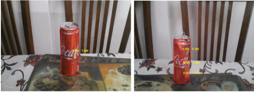
Fig. 3 An ideal can prototype without any deformities (left) and a deformed can to be classified as defective via damage assessment (right)
