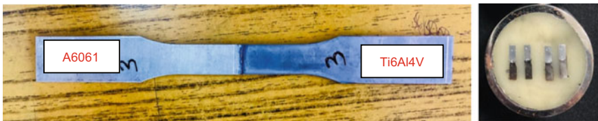
Fig. 4 a Tensile test break sample. b Hardness test specimen
