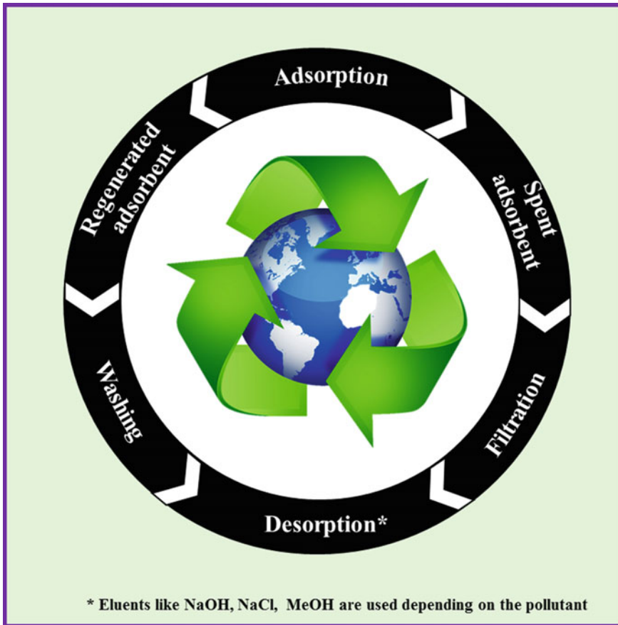
Fig. 3.5 Recycling process for the adsorption technique
