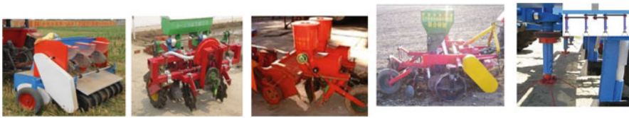
Fig. 25.7 Chinese-modified turbo seeder, powered disc mini-till seeder, powered coultter mini-till seeder, powered straight knife mini-till seeder, powered residue throwing finger no-till seeder
