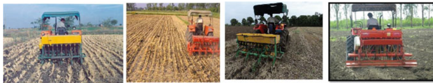
Fig. 25.8 Commonly used zero–/no-till drill, strip-till drill, rotary slit-till drill and bed former cum seeder under CA in India
