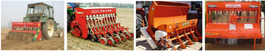
Fig. 25.6 Strip rotary hoe mini-till seeder, strip chop no-till seeder, happy seeder, turbo happy seeder
