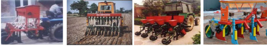
Fig. 25.5 2BMF-7 no-till wheat seeder, 2BMF-11 no-till wheat seeder, 2BMQF-4 no-till corn seeder, and 2BYCF-3 no-till corn seeder
