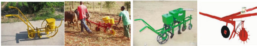
Fig. 25.2 Animal-drawn seeder developed in China, South Africa, India, and Tanzania
