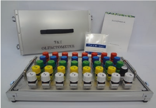
Fig. 25.6 T&T olfactometer [40]. The T&T olfactometer evaluates the detection and recognition thresholds for each of the five odorants. Reproduced from Miwa et al. [41]
