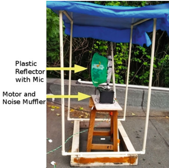
Fig. 3 AED setup with mounting of reflector dish on a motor
