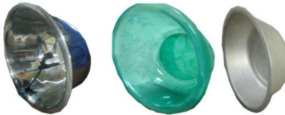
Fig. 2 Acoustic reflectors, steel (dimension: D = 24.2 cm, d = 7.4 cm), plastic (dimension: D = 43.5 cm, d = 13.5 cm) and aluminum (dimension: D = 46 cm, d = 13 cm) (left to right)
