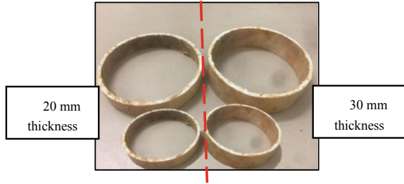
Fig. 4 Mould with diameter of 100 mm and 30 mm for sample preparation
