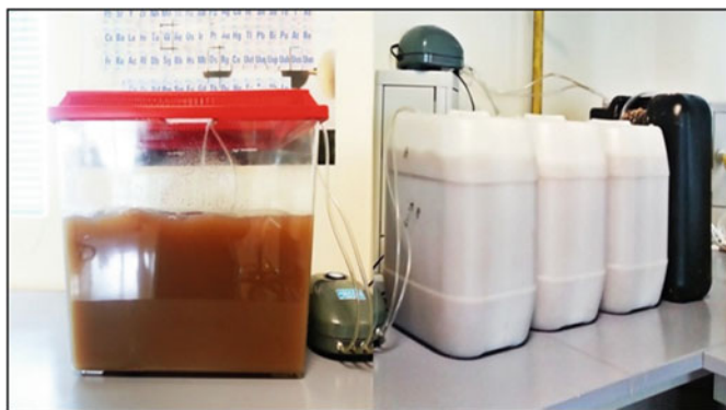
Fig. 1 Activated sludge process of sago effluent
