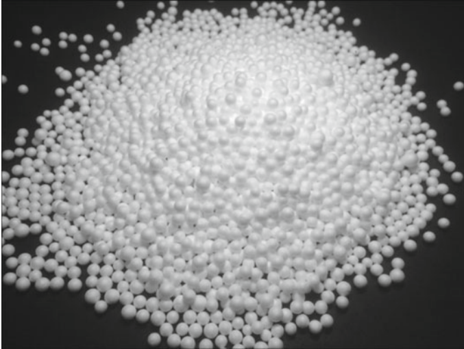
Fig. 4 Expanded polystyrene beads with a size in range of 2.5–4.0 mm
