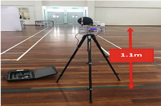
Fig. 3 Placement of thermal comfort kit and its probe
