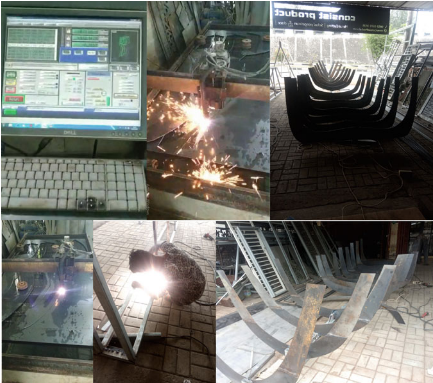
Fig. 19 Manufacturing traditional Aceh fishing boat through metal cutting and welding processes
