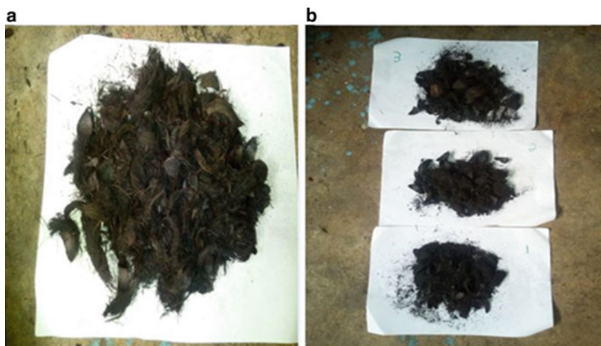
Fig. 4 The images of biochar produced: a without trays and b with trays
