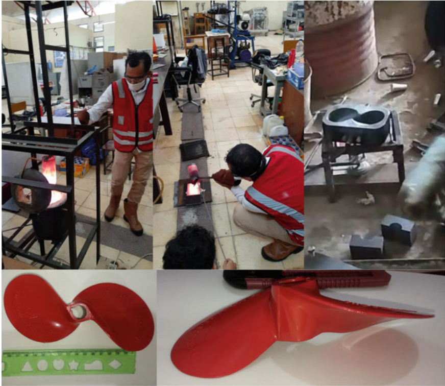
Fig. 9 Manufacturing boat propeller through metal casting processes
