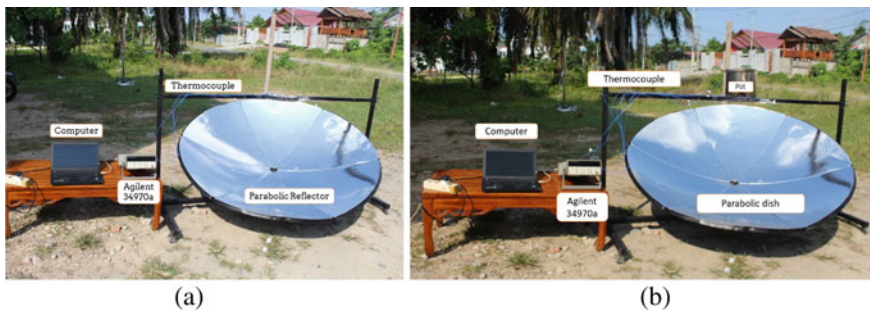
Fig. 2 Solar cooker parabolic dish test a without any loads, b with loads
