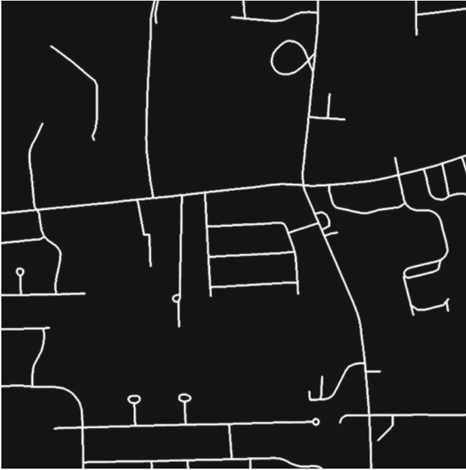
Fig. 6 Annotated sample image. During the training after applying morphology, this image was annotated by marking 1 for lane pixels and 0 for non-lane pixels. This image will be compared with the trained model for measuring the accuracy
