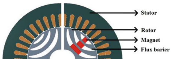
Fig. 12.10 1/4th model of reluctance synchronous motor and ferrite-assisted reluctance synchronous motor
