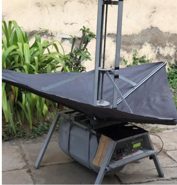
Fig. 1.1 Real-time model of intelligent stand-alone solar PV-enabled rainwater collector and power generator
