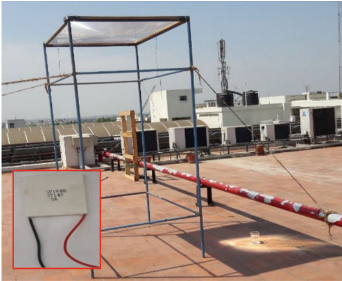
Fig. 1 TEG experimental setup with Fresnel lens
