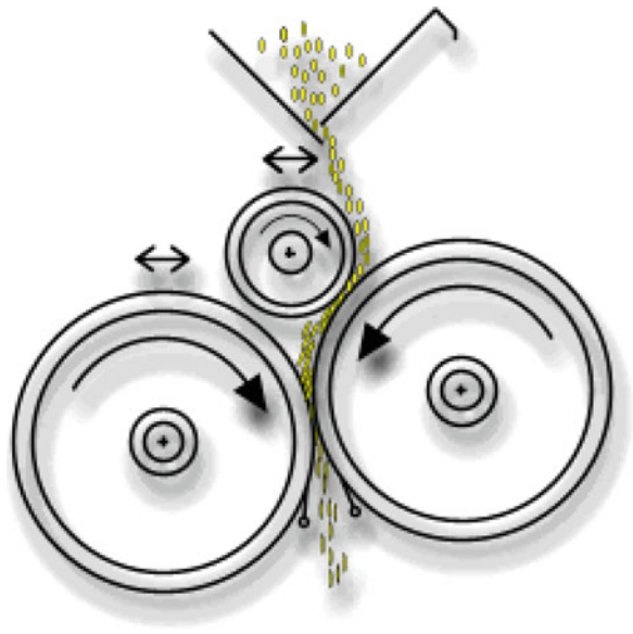
Fig. 11.1 Typical roller mill
