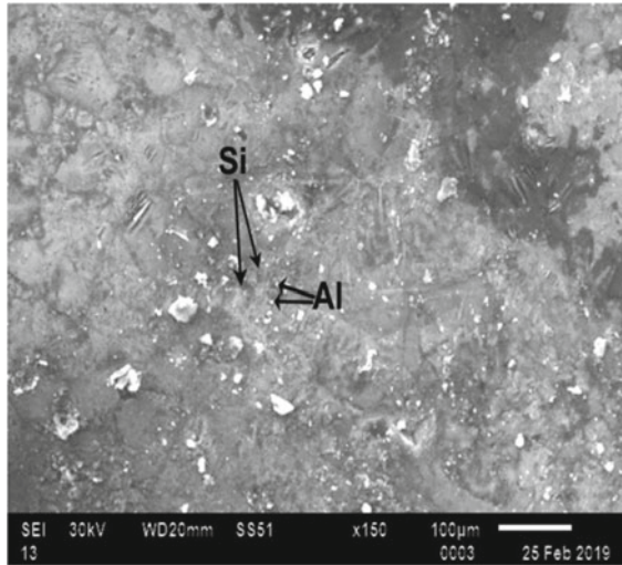
Fig. 8 SEM microstructure of UVSS-T6-casted AlSi24 alloy
