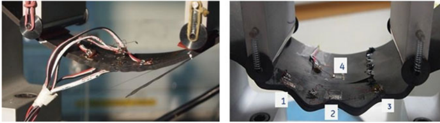
Fig. 2 Case 3 and case 19 type coupons under 4-point bend configuration
