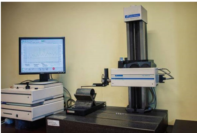
Fig. 2 Set-up for ‘Talysurf’ roughness tester
