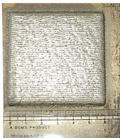
Fig. 1 LDED of Hast-X a setup; photographic view of b bulk deposit and c cross-sectional microstructure
