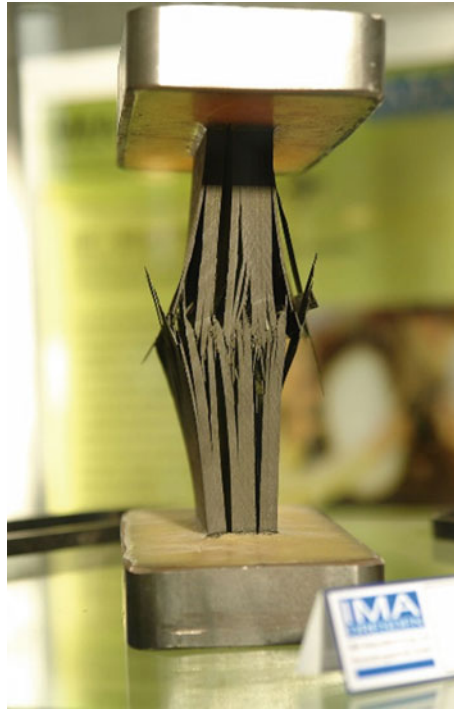
Fig. 7 Delamination of carbon fiber reinforced polymer under compression load [Courtesy: Wikimedia Commons (under free reuse license)]
