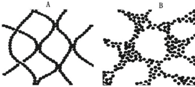
Fig. 3.10 Schematic diagram of network structure of protein gels. a Orderly aggregation; b Free aggregation
