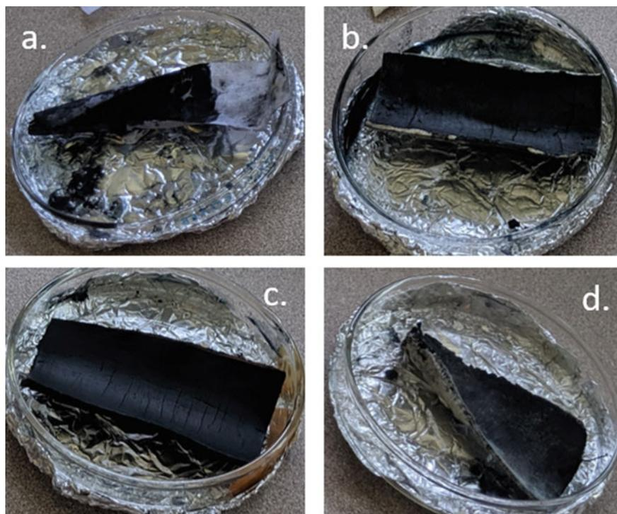
**Fig. 9** Different fabrics coated with a polypyrrole paste: **a** nylon, **b** chamois, **c** leather, and **d** canvas
