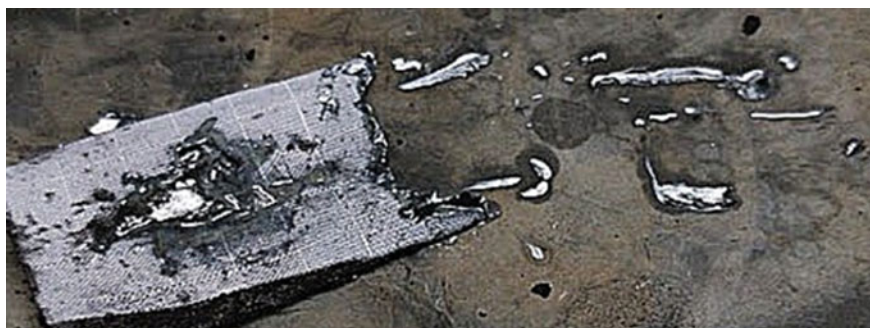
Fig. 13 Nylon anode melted away after improper \text{TiO}_2 paste coating
