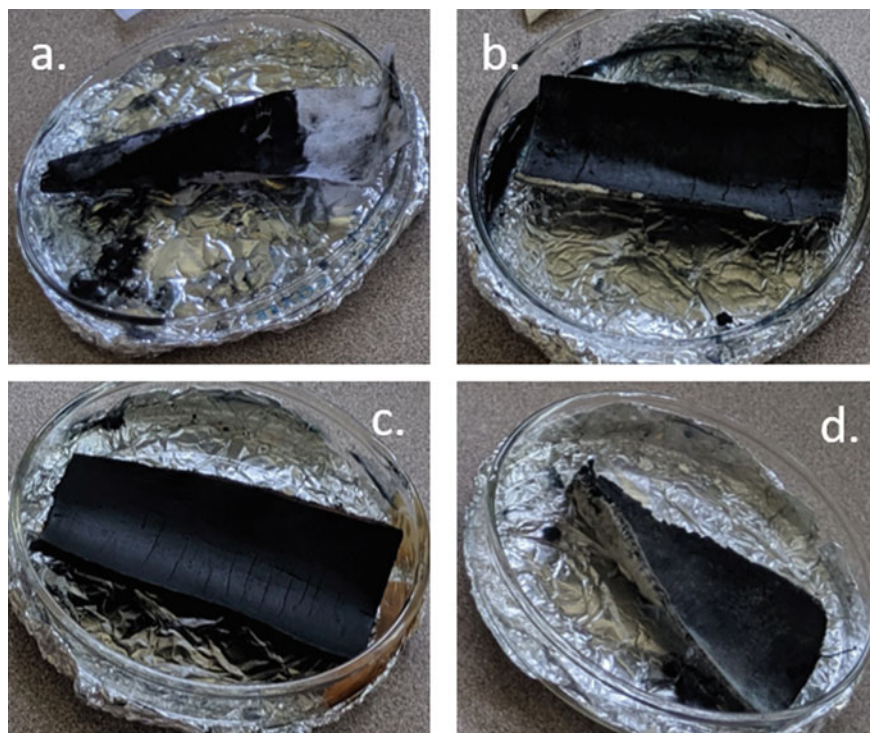
Fig. 9 Different fabrics coated with a polypyrrole paste: a nylon, b chamois, c leather, and d canvas
