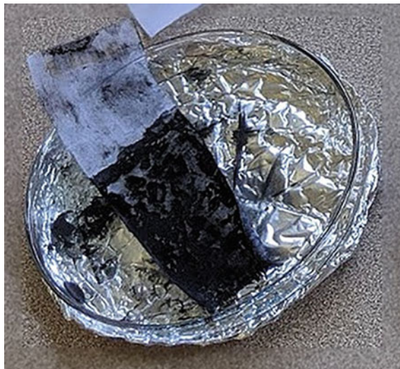
Fig. 10 Coating of polypyrrole on the textile over time: a prior, b after a day has passed, showing mild to severe cracking on the surface
