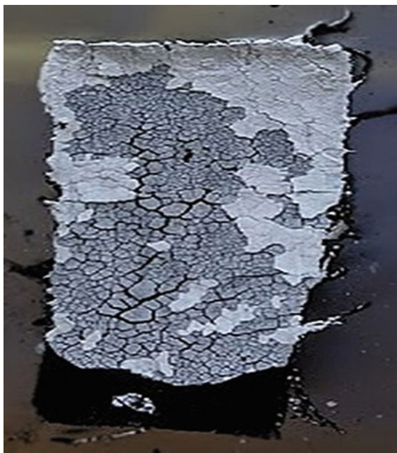
Fig. 12 Fragmented, cured \text{TiO}_2 paste peeling off from the coated canvas fabric
