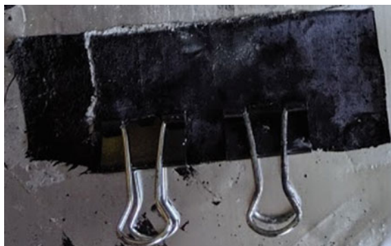
Fig. 16 Assembled TDSSC cell held together by binder clips before the application of the electrolyte
