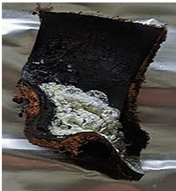
Fig. 14 Leather anode burnt and contorted after improper \text{TiO}_2 paste coating
