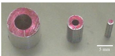
(a) A nest of test jigs for spatial resolution measurement. The right cylinder was used for the measurement.
