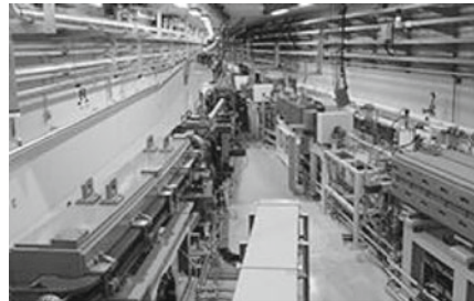
(b) Beam injection section into the storage ring (right) from the beam transportation line (right)
