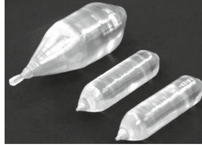
(b) LuAG (Pr) ingots grown by the Czochralski method
