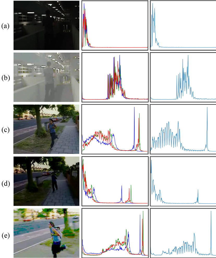
Fig. 4. Comparison of sampled frames and the RGB (middle column) and Y (right column) value histograms of their corresponding videos from (a) ARID, (b) ARID-GIC, (c) HMDB51, (d) HMDB51-dark and (e) HMDB51-dark-GIC datasets. GIC enhancement shifts the RGB and Y value histograms towards the larger values, indicating brighter video frames. The RGB and Y values of ARID and ARID-GIC are more concentrated than that of HMDB51-dark and HMDB51-dark-GIC respectively, which matches the low contrast and pale sampled images. The peaks of the RGB histogram at the higher values of the HMDB51-dark video comes from the bright background. Best viewed in color and zoomed in. (Color figure online)
