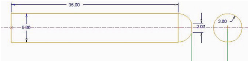
Fig. 1 Geometry of pin specimen
