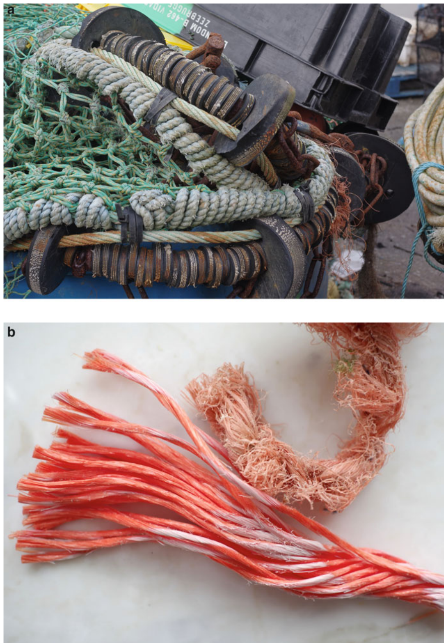
Fig. 14.2 The fishing nets (a) in the harbour and (b) in the laboratory and their changes during weathering under the UV radiation
