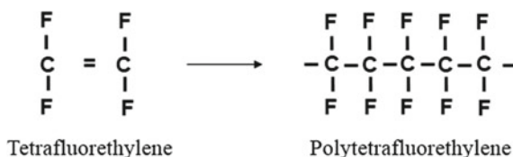
Fig. 33 Chemical structure of polytetrafluoroethylene (PTFE)
