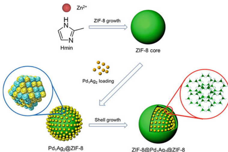
Fig. 9.7 Schematic illustration for the synthesis of ZIF-8@PdAg@ZIF-8
