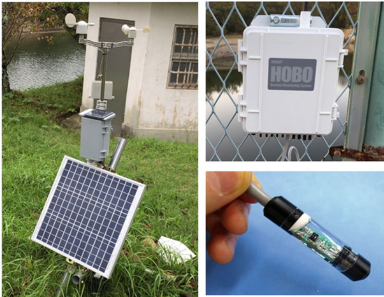
Fig. 7.4 Weather station (left), data logger (upper right), water level sensor (lower right)
