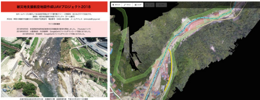
Fig. 4.3 Website of UAV mapping project (left) and photogrammetry map by drone (right)
