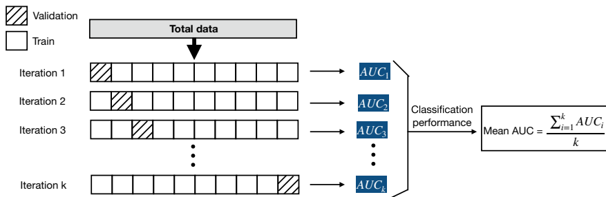
Fig. 3 Process of classification performance evaluation based on SVM and k -fold CV. The figure is original.
