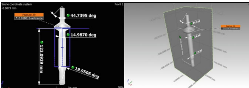
Fig. 18 Slice views with some dimensional measurements made on poppet of fuel injection valve
