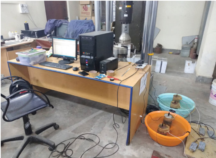
Fig. 1 Accelerated corrosion test setup using AE monitoring system in Structures Laboratory, Department of Civil Engineering, Indian Institute of Science, Bangalore, India
