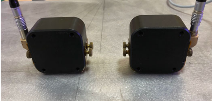
Fig. 4 EMAT probes placed on aluminum sample of 2 mm thickness. Distance between the probes is 143 mm
